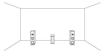
Center placement against the front wall is often optimum for music or movie systems where the subwoofer is used to reproduce left/right channel bass. It provides high output and good "imaging".
